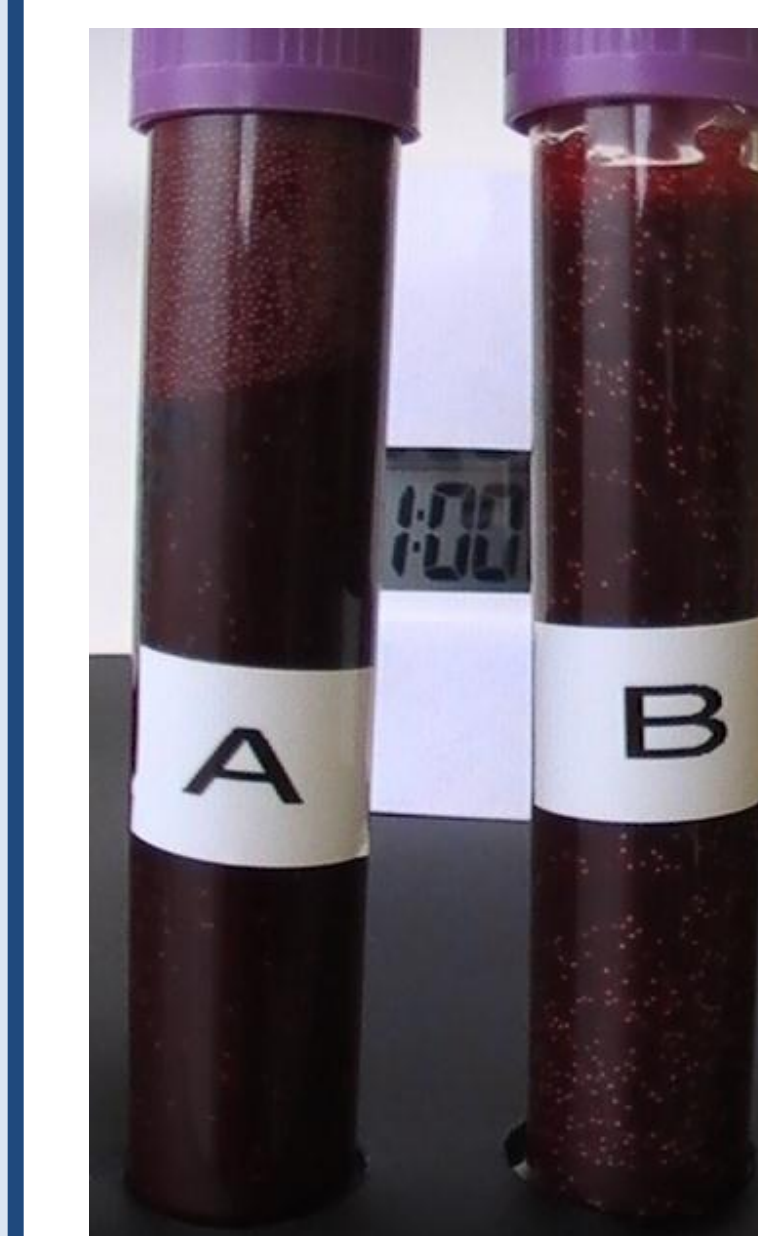
Fig. 2: Neutrally-buoyant beads (right) versus normally buoyant beads (left) after incubation for 1 hour in pRBCs
